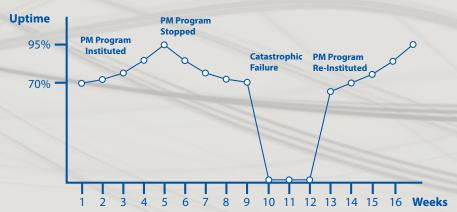
An example of the effectiveness of preventive maintenance is shown in the graph above. This is an actual example of the effect of preventive maintenance for a key piece of equipment in a factory in the aseptic packaging industry. It vividly demonstrates the worth of an effective preventive maintenance program.
